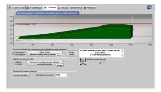
for a more complete analysis should be used "multiple analysis" which offers many views of performance and test options. For example when the propeller is coupled to an electric motor or a generator, the actual rotational speed of the propeller will be the one which balances the engine torque and the load torque. To determine how fast the spin system, it is easier to make a superposition of torque curves, according to the rotational speed with multiple analysis.
