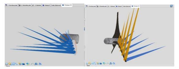
Directions Lift - pusher propeller thrust (left) and lift-torque wind turbine (right)
