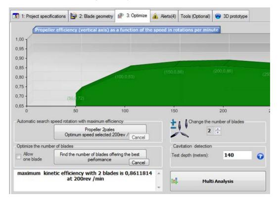
A quick search of optimum speed, for a given geometry can be executed from the tab "optimize". If you wish, HELICIEL automatically calculates the speed offering the optimum performance of a propeller you have determined the geometry. If you wish, HELICIEL automatically calculates the speed offering the optimum performance of a propeller you have determined the geometry.
