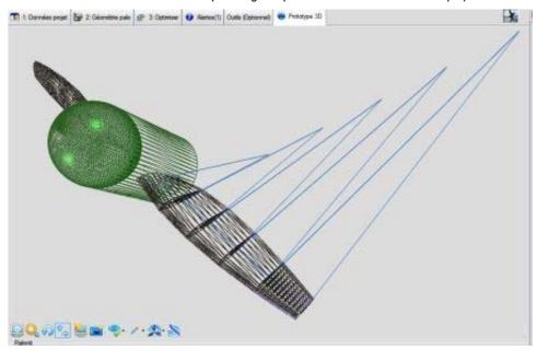
Apparent wind vectors for each element in **HELICIEL**
